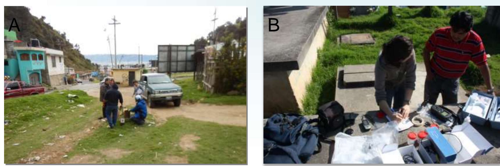
Fig. 7 – (A) Water level measurements in a well in Quetzaltenango. (B) Water sampling from municipal collection tanks and data-gathering
